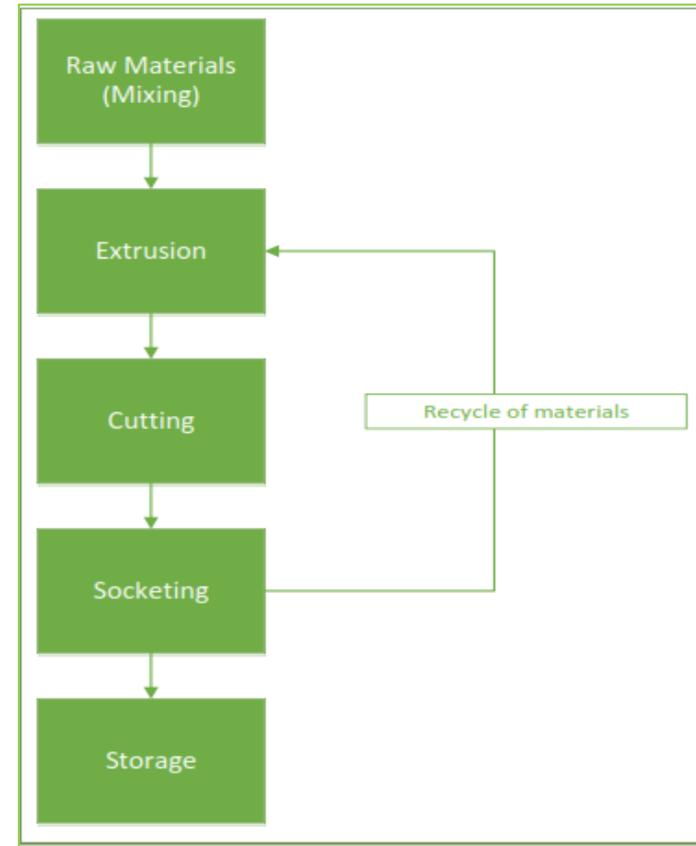
**Example Process Flow Diagram**
